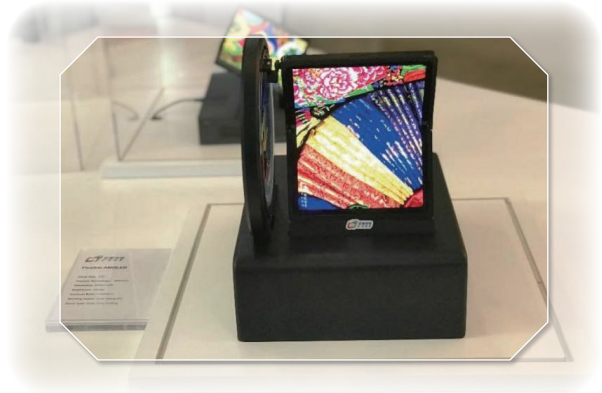
7.2-inch OLED flexible foldable screen
